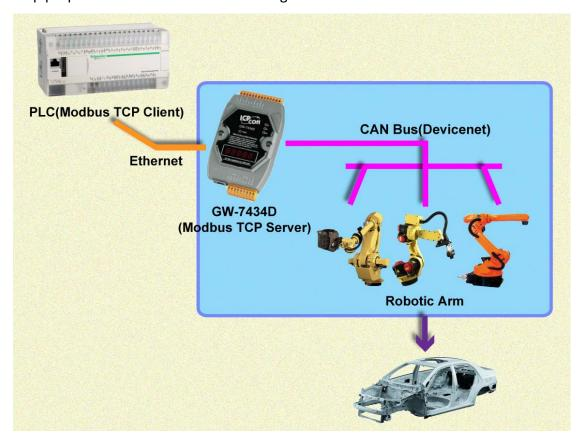
The customer use PLC which has Ethernet interface and Modbus TPC protocol to control robotic arm with DeviceNet protocol for moving and to polishing vehicle body.
